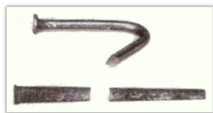
Fig. 17.1.2 Soft, low-carbon steel bends easily while hard, carbon-rich steel breaks instead of bending.
