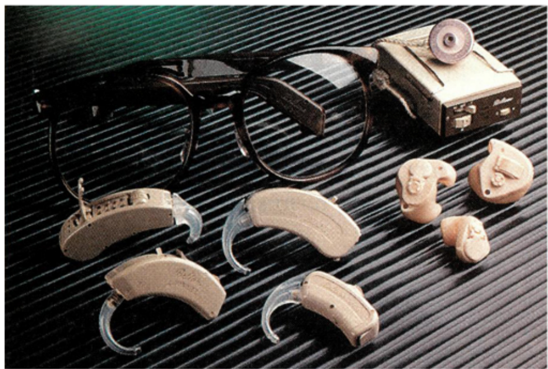
FIGURE 10-12 Hearing Aids Worn by people with conduction deafness, hearing aids send sound impulses through the bone of the skull to the cochlea.
